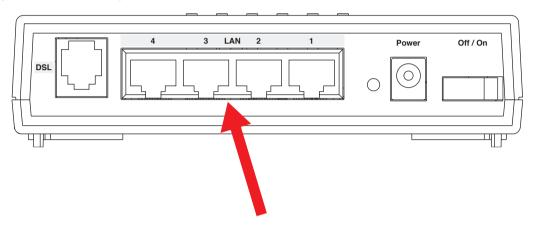
If you add devices connected through a hub or switch, connect the hub or switch to an Ethernet port on the Netopia 4-port ADSL Router.
